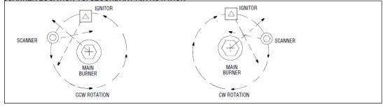
5. Having determined the approximate location for the sight pipe, cut a clearance hole for a 2 inch pipe through the burner plate. Look through the hole. If register vanes interfere with the desired line of sight, the interfering vane(s) should be trimmed to assure an unrestricted viewing path at all firing levels as indicated in Figure 6.
