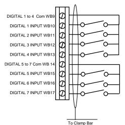
These Low Voltage digital inputs can be used for safety related functions and their function is programmed by option parameters 68.1 to 68.7 inclusive.
