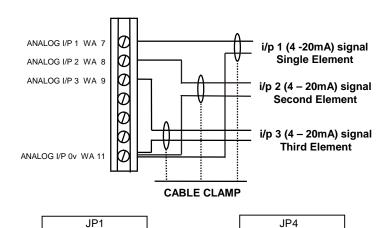
The pressure sensor cabling MUST be overall 'braid' screened PVC insulated 7/0.2mm (number of cores as required by the relevant sensor). As this cable may lay adjacent to, and/or in the same conduit as Line voltage wiring, the cable voltage rating must exceed the maximum voltage carried by any other cable connected to the controller or run in the same conduit.
