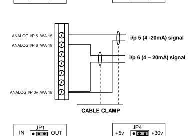
Connect the cable 'braid' screen to the controller with the use of the screen termination clamp. Make all connections at the sensor/transmitter first.
