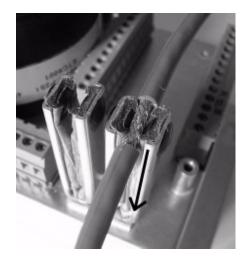
Where screened cables are required to run through one device to connect to another, terminals are provided to allow the screens to be connected, by forming a 'tail' with the braided screen of each cable, the length of unscreened cable short be kept as short as possible, but in any case **MUST NOT exceed 30mm**, per cable 'tail'.
