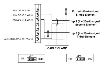
The pressure sensor cabling MUST be overall 'braid' screened PVC insulated 7/0.2mm (number of cores as required by the relevant sensor). As this cable may lay adjacent to, and/or in the same conduit as Line voltage wiring, the cable voltage rating must exceed the maximum voltage carried by any other cable connected to the controller or run in the same conduit.
