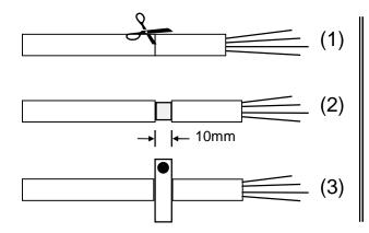
The cable should be prepared by cutting around the outer insulation, taking care not to damage the screen (1).
