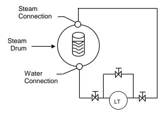
Typical Level Transmitter Piping
