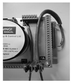
Route the screened signal cables through the clamps, exposing the braid in the clamp, before terminating at connectors.
