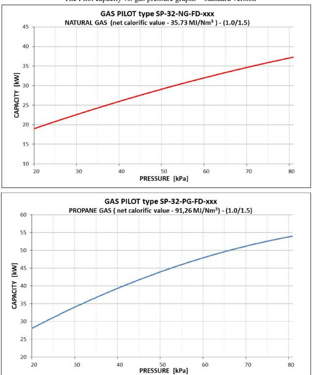
The Pilot capacity vs. gas pressure graphs - standard version
