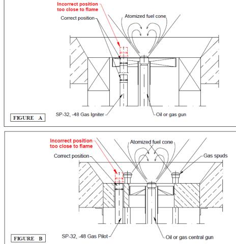
Gas Igniter operating as an intermittent (light-off) on a sample single gun main burner, oil or gas fired, vertical or horizontal mounting.
