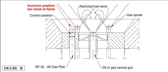
**Fig. A** Typical for power & utility boilers, industrial heaters - shows position of **SP-32** and **SP-48** Gas Igniter operating as an intermittent (light-off) on a sample single gun main burner, oil or gas fired, vertical or horizontal mounting. The pilot air tube tip can reach the swirler or can be placed before it. Pilot tip cannot extend beyond the swirler plane.
