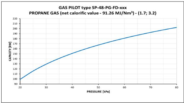
Remark: The real measured capacity may differ by  $\pm$  5% depending on a particular pilot and measurement conditions
